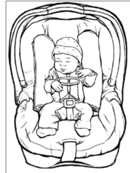
Figure 2: Car safety seat with a small cloth between crotch strap and infant, retainer clip positioned at the midpoint of the infant's chest, and blanket rolls on both sides of the infant.
